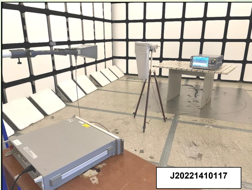
Photo 6: Test Setup Without Test Sample
